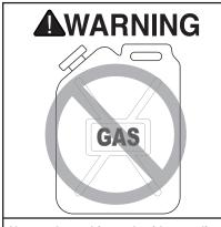
Never clean this tool with gasoline or other flammable liquids. Vapors in the tool may ignite, causing the tool to explode. Ignoring this warning may lead to serious personal injury or even death!
